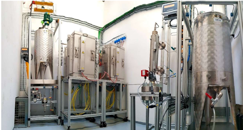
Pilot-scale hydrotreater (24/5 operation – 50 kg/day)
