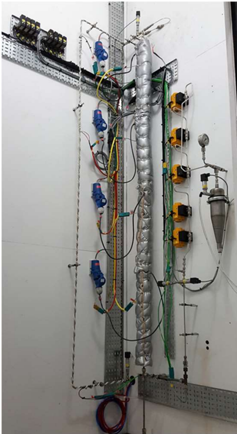
Bench-scale hydrotreater (24/7 operation – 1 kg/day)
