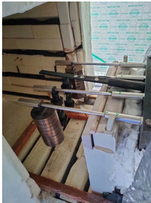
Figure 1: Samples of Experiment 2 in the test furnace before starting the creep bending test.
