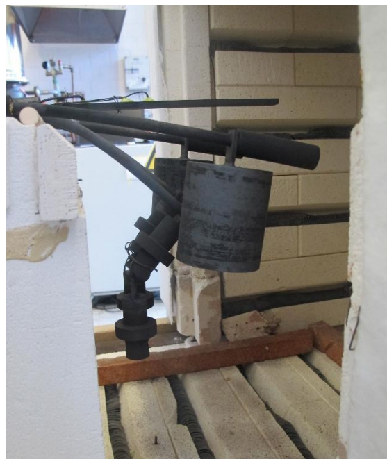
Figure 11: Experiment 2 creep bending samples after 100h at 900°C.
